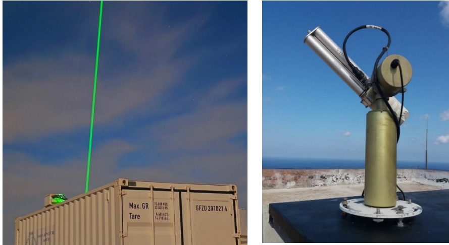
Figure 3 The Polly XT ground-based Lidar (left) and the CIMEL sun photometer located at PANGEA station (right).
